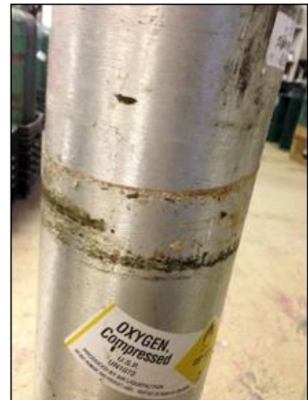
Contaminated cylinders, valves and connections
