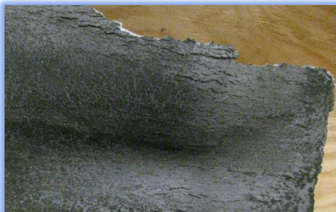
Example of stress crack corrosion on the inside of a cylinder containing CO and CO 2 .
