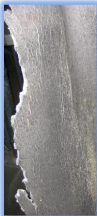
Example of stress crack corrosion on the inside of a cylinder containing CO and CO 2 .
