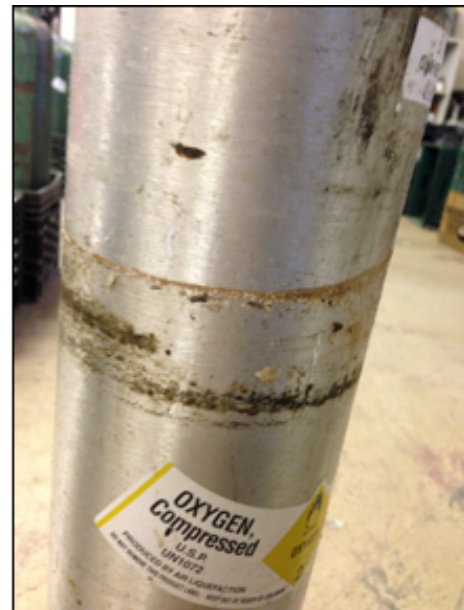
Contaminated flood water line
