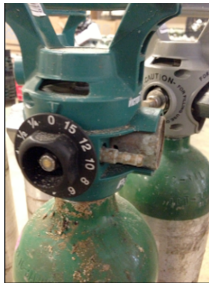
Contaminated valves & connections
