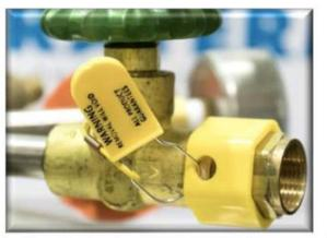
Non-Compliant - This valve outlet connection can be removed with scissors
