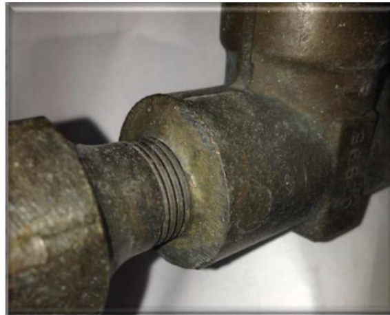
This valve outlet connection is permanently silver-brazed
